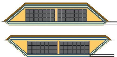
Figure 1: Suggested surface (upper), or a near surface (lower) concept for the LILW disposal facility
